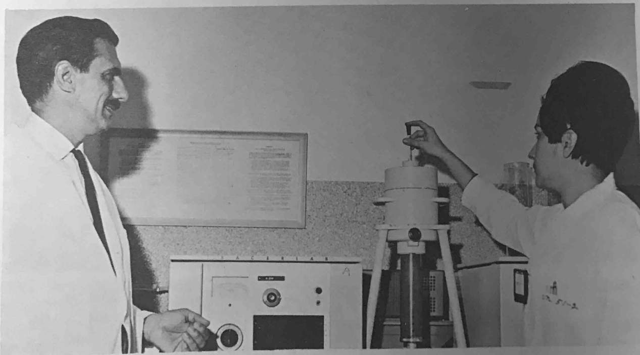
Measurement of a fluid sample in a well counter.
