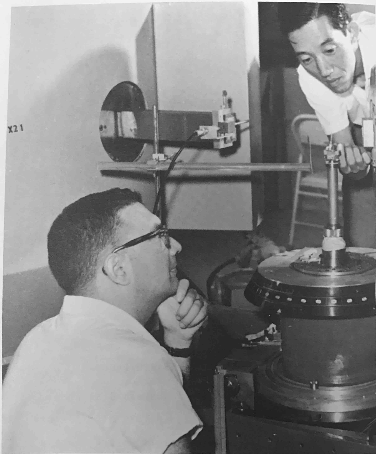
Dr. M. I. Kay (left) and Dr. K. Okada check the final mounting of a crystal on the goniometer installed on PRNC's automatic neutron spectrometer.
