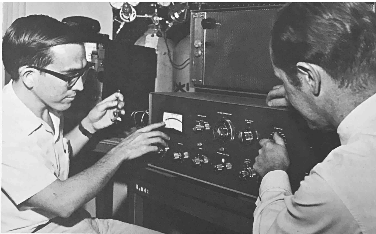
Dr. Manfred Eberhardt and Mr. Alfonso Mata, a student from Costa Rica, operating a vapor phase chromatograph.
