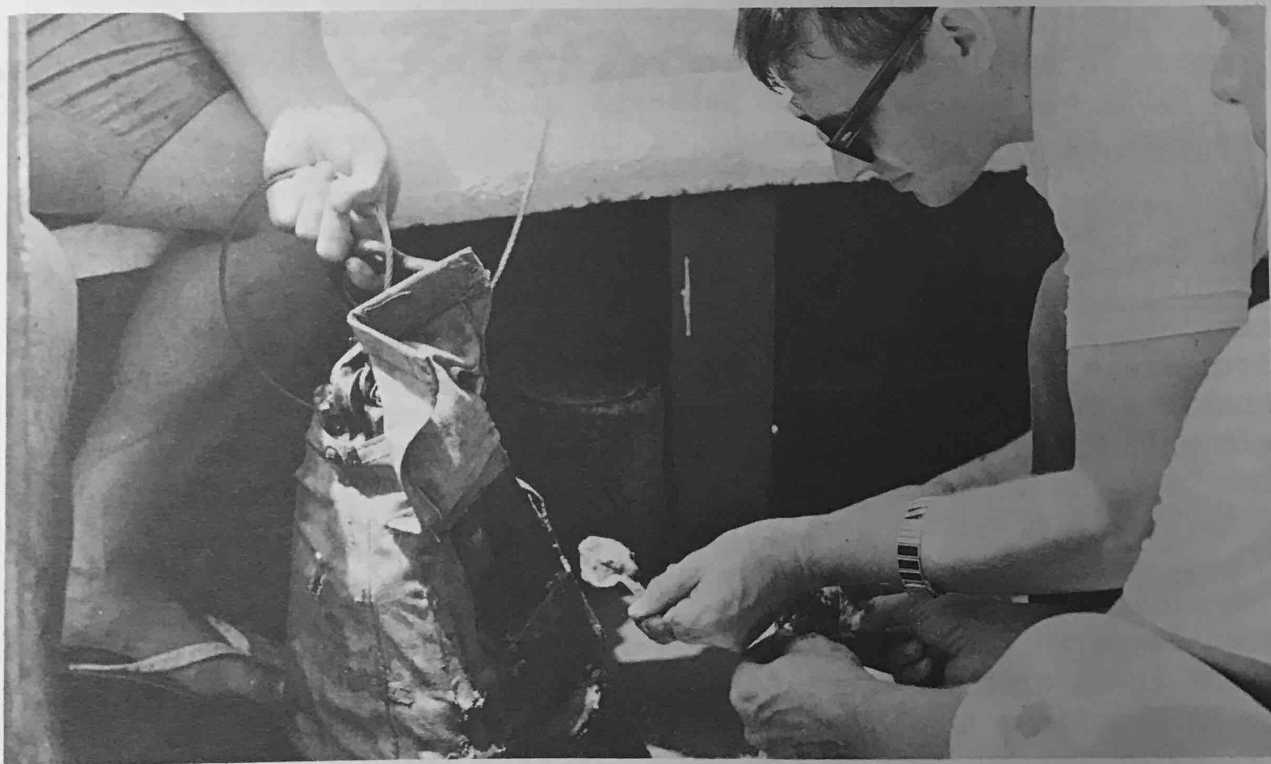
Dr. R. Gordon Pirie removing a sediment sample from the orange-peel-grab.
