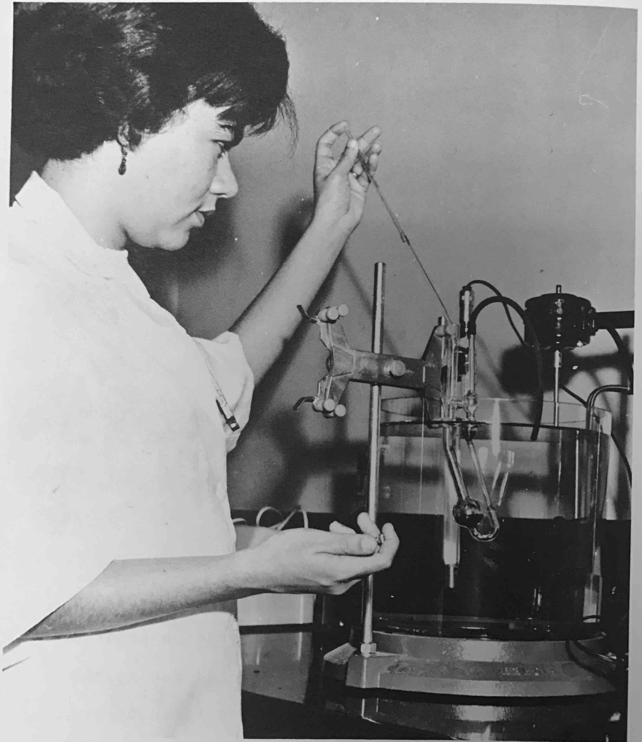
Technician C. Asencio determines the weight average molecular weight of pectins by viscometry.
