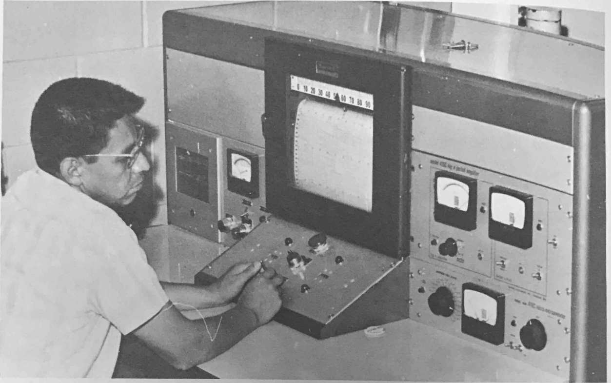
Above: Control rods are adjusted before transfer function measurement on the L-77 reactor. Below: Transfer function measurement experiment on the L-77 reactor.
