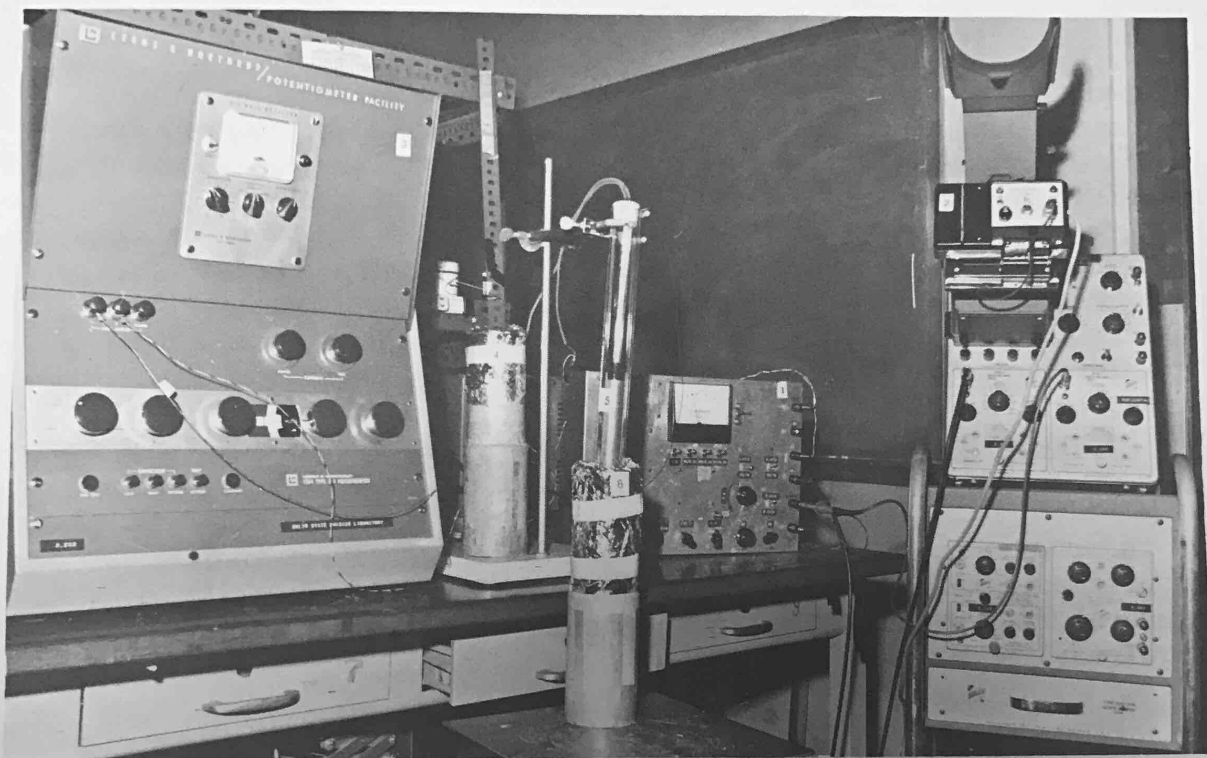
Scope and camera used for hysteresis loops measurement in ferroelectrics at low temperatures.
