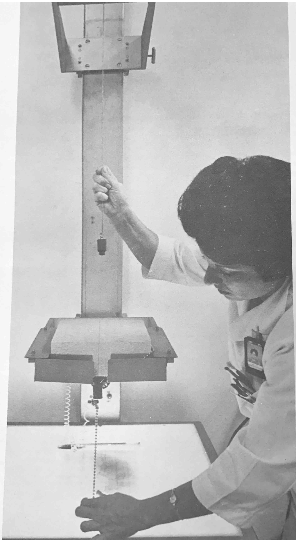
This styrofoam poly-shaper is used for making styrofoam molds in which blocks will be formed to shield critical areas of the body during radiotherapy. From a block of styrofoam a portion of the required shape is cut by wire, heated by an electric current. The shape of the styrofoam removed is determined by moving a pointer held at the lower end, over an illuminated radiograph on which the required shape is marked. The equipment is being manipulated by Miss Cecilia Ramirez, a dosimetrist in the Medical Physics Section.
