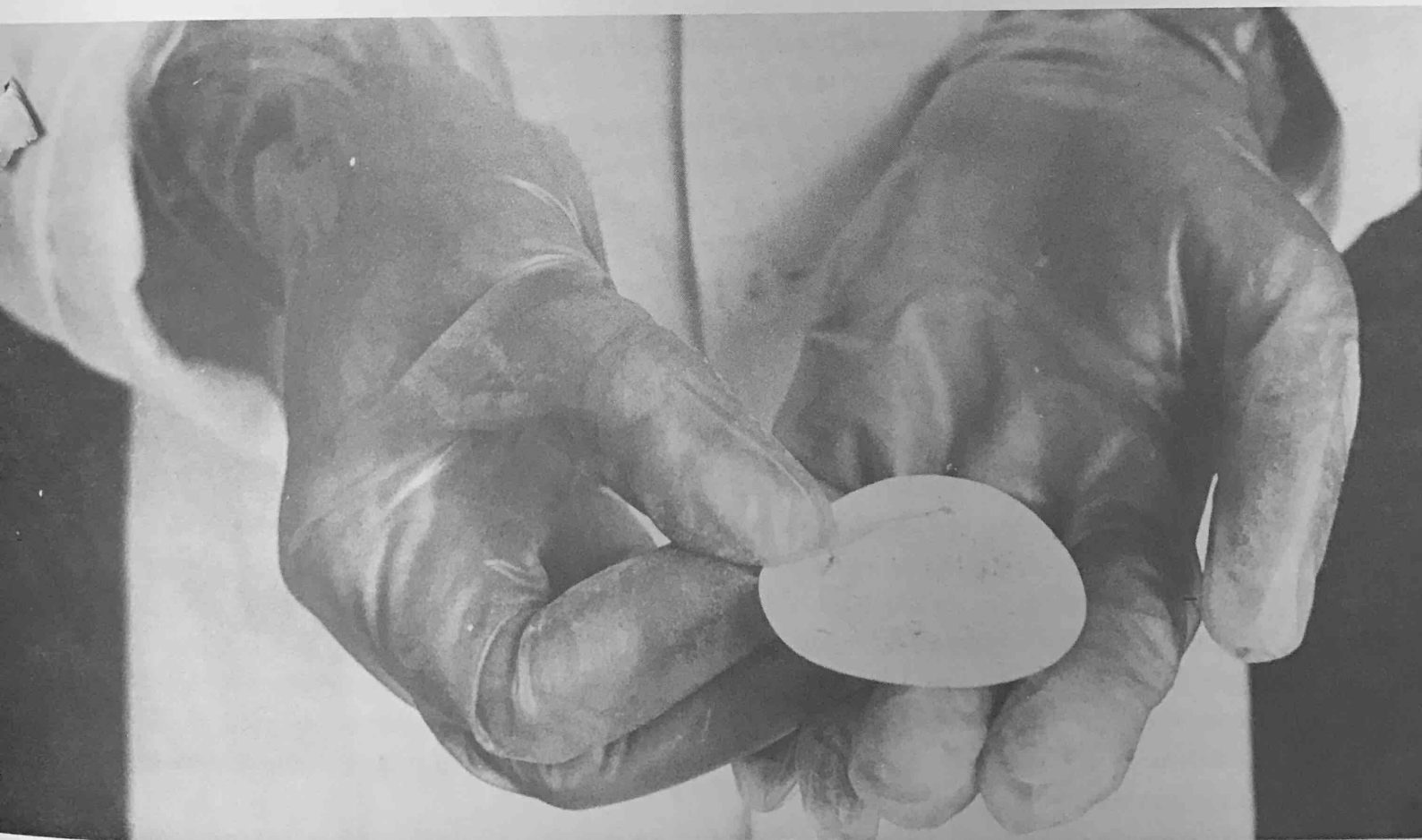
A smear taken in one of the laboratories to detect radionuclide contamination.
